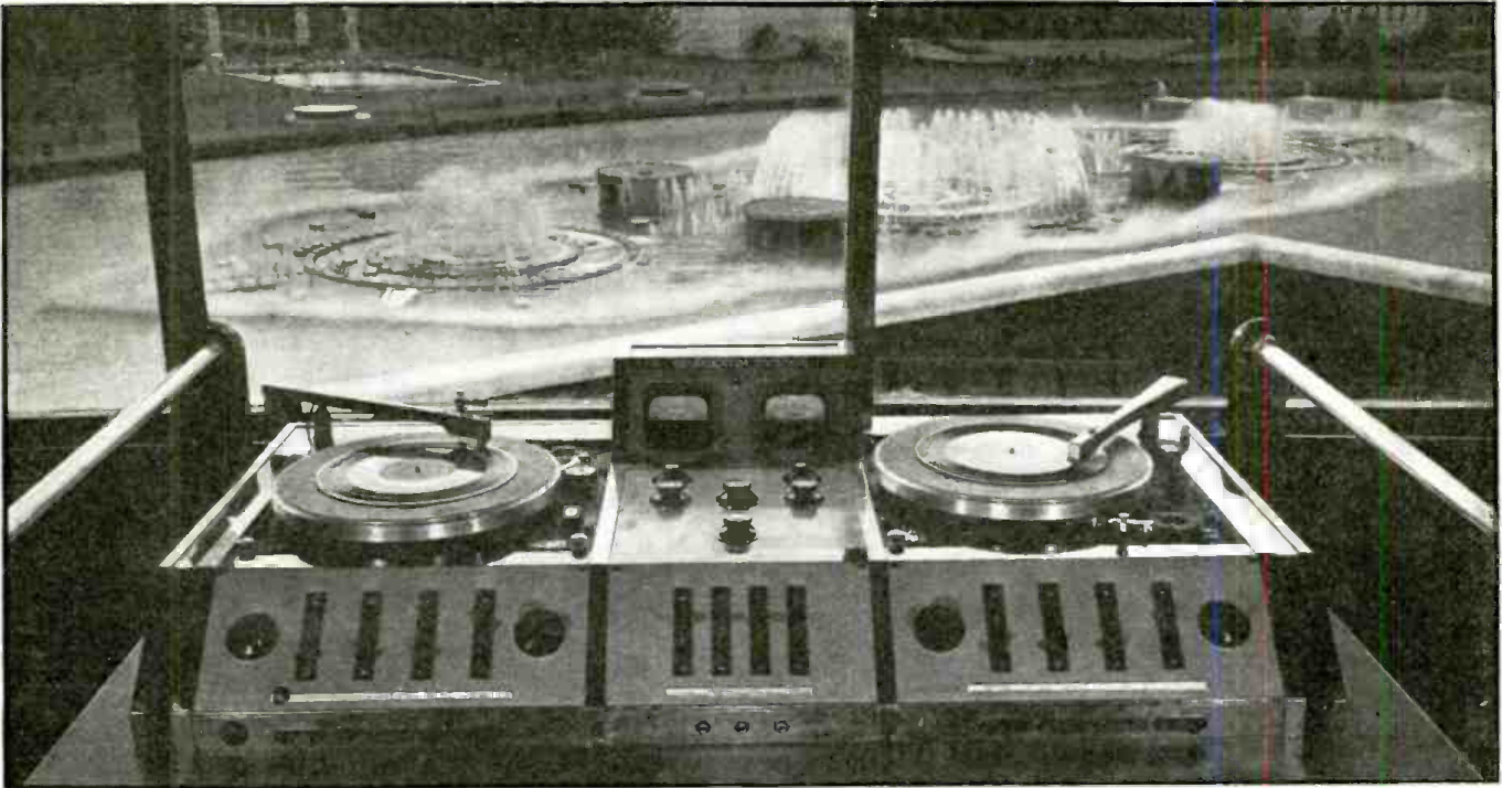
You're looking at the extravaganza of sound, fire and water at the New York World's Fair, through the windows of the "cue" (control) room atop the Rumanian Pavilion. Twenty tons of water, 2,000 watts of sound, 1/2-million cubic feet of gas and many rounds of fireworks are all controlled from this nerve center.
