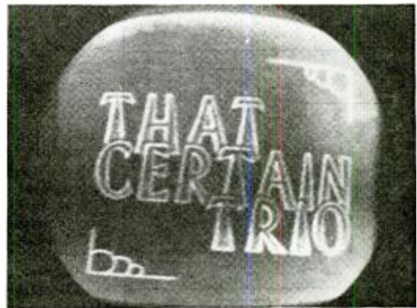
▲ Fig. 10. This photo depicts the uneven image illumination resulting from inadequate low-frequency response.
